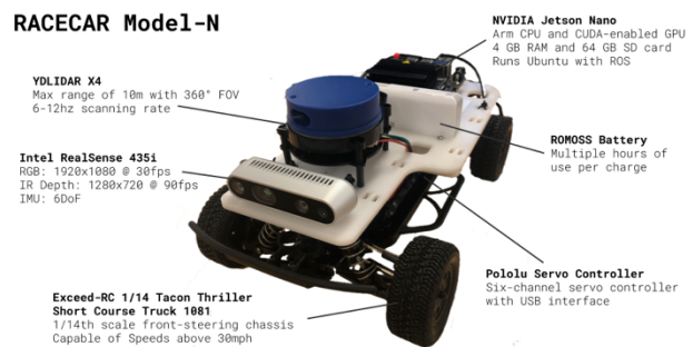
Figure 1. RACECAR-N with most important components highlighted.
